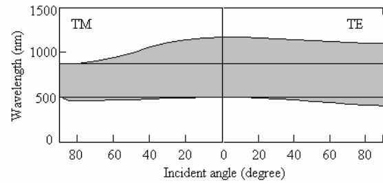
Fig. 6. Photonic band structure of combination of Fibonacci quasi-periodic and periodic structures.
